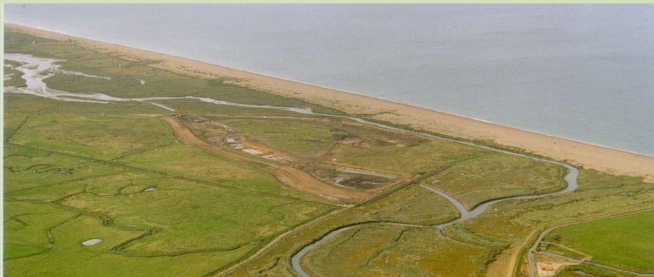
Photo 3: River Glaven realignment under construction behind the Cley to Salthouse shingle barrier
