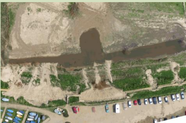
Photo 3: River Glaven realignment under construction behind the Cley to Salthouse shingle barrier
