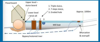
The RRC were asked by the National Trust to provide a management options assessment for Coleshill Mill, Wiltshire. A leat was constructed to provide water to the mill and in the 1990s, restoration of the natural river course took place to divert the majority of flow away from the mill building to protect it from flooding. Now, the mill is used for demonstrations, but staff have found that operation of the mill has become increasingly difficult due to a reduction of flow.
