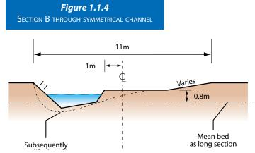
The stiff clays in the river banks resisted erosion preventing cliffs from forming on the outside of meander bends where 1:1 batters were cut. Conversely, floodwaters were racing across the flat areas formed on the inside of each meander causing scour of the surfaces. The asymmetrical profiles were subsequently re-excavated as indicated on Section B.
