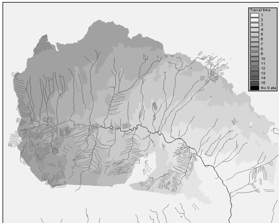
Figure 5. Map of grip locations in the Oughtershaw sub-catchment of the Upper Wharfe, North Yorkshire. This is superimposed to a map of predicted catchment travel times to emphasise that grips don't simply affect the partitioning between overland flow and subsurface flow; they also affect the relative timing of flow delivery.
