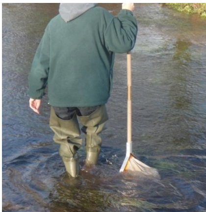
Figure 2: Kick sample and Surber sample methods
