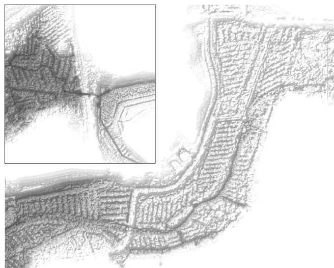
Figure 10.1 An example of LiDAR data, showing fine details of a derelict water meadow system on the River Nar SSSI in Norfolk (© Environment Agency copyright 2010 and the River Restoration Centre).
