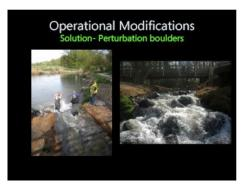
Solution- With assistance I placed a combination of gabion rocks and larger 300-450mm perturbation boulders (Heimerl & Wurster 2006) in to the entrance of the pass and the first riffle to baffle the flow, producing areas of slack water for fish to rest in whilst ascending into the pass.
